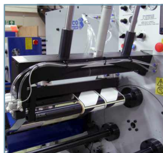
3 Position turret with mandrel end support
